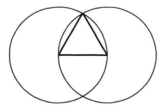
Describe a circle. With unaltered compasses describe a second circle, using any point on the circumference of the first circle as the center of the second. The space enclosed by the intersecting lines of the two circles is
